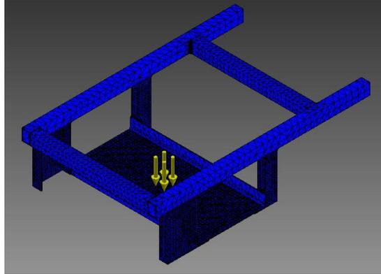
**Figure 2.** The image shows the constraints and loads applied to the frame for the finite element analysis. The constraints model the four wheels that limit vertical displacement. The load represents the weight of the batteries, the dominant force expected for static loading.
