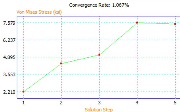
**Figure 3.** Convergence plot for the finite element analysis of the frame. The software successfully converged the Von Mises stresses to within 1.1% with a mesh of 128,000 elements.
