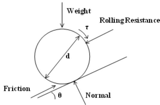
**Figure 4.** Free body diagram of vehicle tire on an incline
